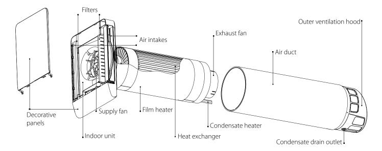
During the operation of the unit, the air flows through the heat exchanger located in the work module. This allows the exhaust air to transfer heat to the cooler supply air, ensuring high quality ventilation.
