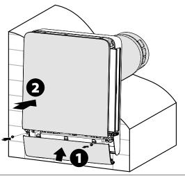
9. Open the air intakes before switching on the system. If the air intake is not open and the product is running, it may damage the unit and cause it to malfunction.
