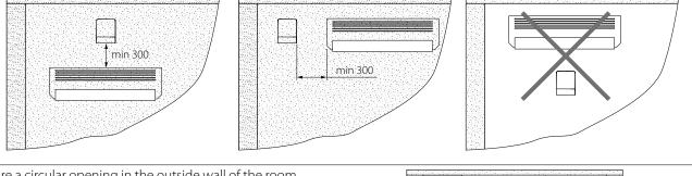
2. Prepare a circular opening in the outside wall of the room with a minimum diameter of 162 mm for Breezy 160-E and 206 mm for Breezy 200-E, sloping downwards towards the street.
