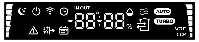
The digital segment of the display shows information such as time, temperature, humidity or all of them in sequence. You can also select the temperature sensor to display (outdoor, supply air, indoor) and select a CO<sub>2</sub> or VOC sensor. The scale on the right shows the fan speed. The scale on the left shows the air quality.
