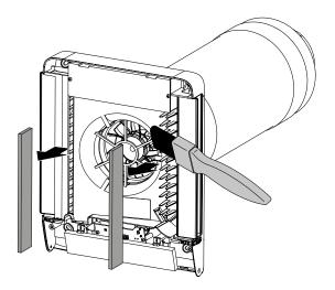
Remove the front panel from the work module. Disconnect the cable and wires. Remove the cover. Unscrew the four screws holding the indoor unit, then remove it from the air duct.
